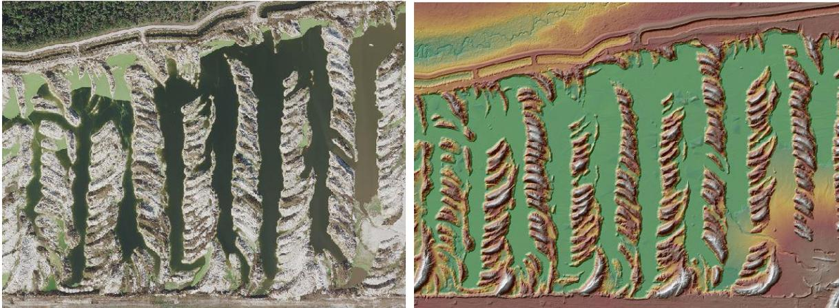
Figure 13 – LID2017\_476018\_W. Orthoimagery (left) of a phosphate mining area and corresponding DEM (right). These locations were classified in the lidar as class 1: unclassified and class 2: ground.
