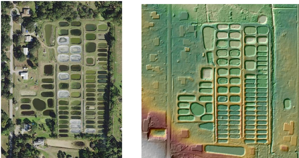
Figure 12 – LID2017\_472713\_W. Orthoimagery (left) of a tropical fish farm and corresponding DEM (right). These small ponds were classified in the lidar as class 1: unclassified and class 2: ground.
