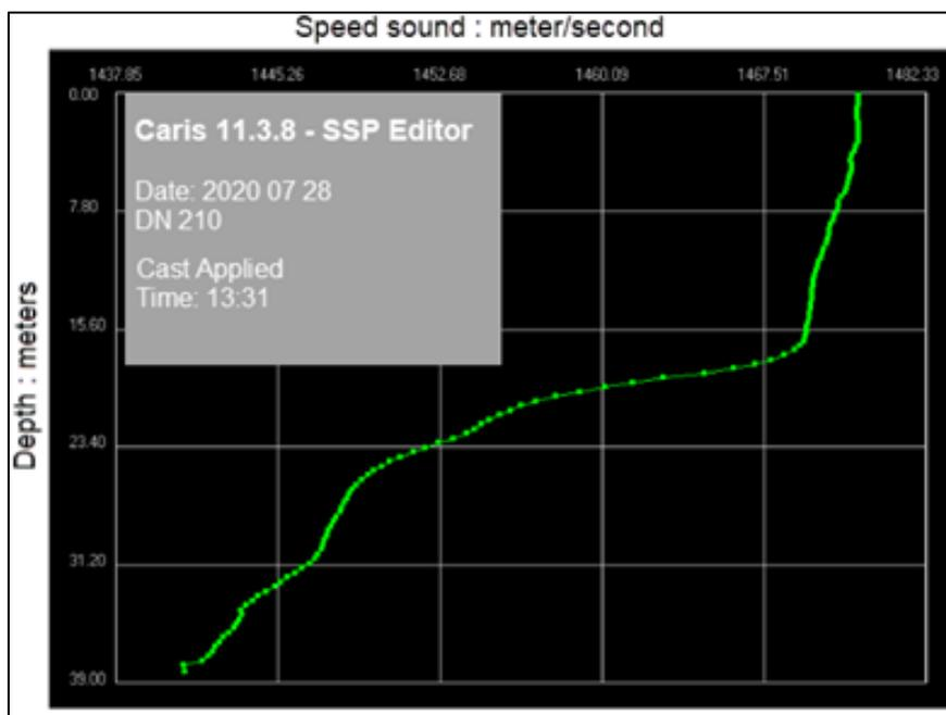
**Figure 6** Example sound speed profile acquired on 7/28/2020 during survey operations. Underwater sound speed varies from approximately 1475m/s near the surface to approximately 1445m/s near the lake bottom at a depth of approximately 39m.
