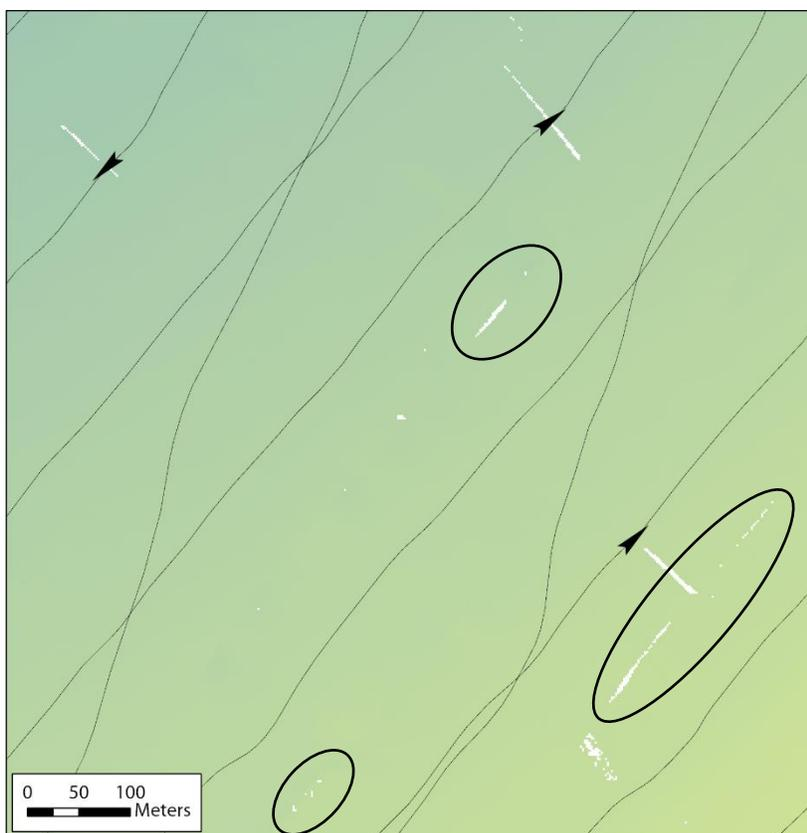
**Figure 5** Along- and across-track data gaps in multibeam data set. Across-track data gaps frequently occurred between individual multibeam sonar files; black lines are survey tracklines with arrows indicating start/stop point between individual sonar files. Along-track data gaps, indicated by black circles, were less frequent and generally due to insufficient overlap between adjacent sonar swaths.
