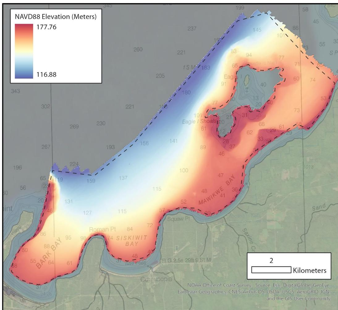
**Figure 3** Multibeam bathymetry surface (2m grid resolution) for Areas 1-3 with multidirectional shading applied. Black dashed line indicates boundary of survey area. Background is NOAA chart 14966 with soundings shown in feet relative to Lake Superior Low Water Datum (601.1 feet).
