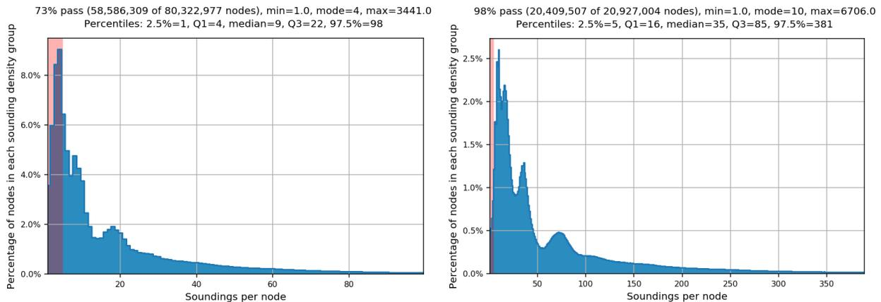
**Figure 1** Density analysis results for 1m bathymetric surface (left) and 2m bathymetric surface (right) with summary statistics. Red shaded region indicates nodes with <5 soundings. Note change in scale of horizontal axes. The 1m bathymetric surface did not meet sounding density requirements.
