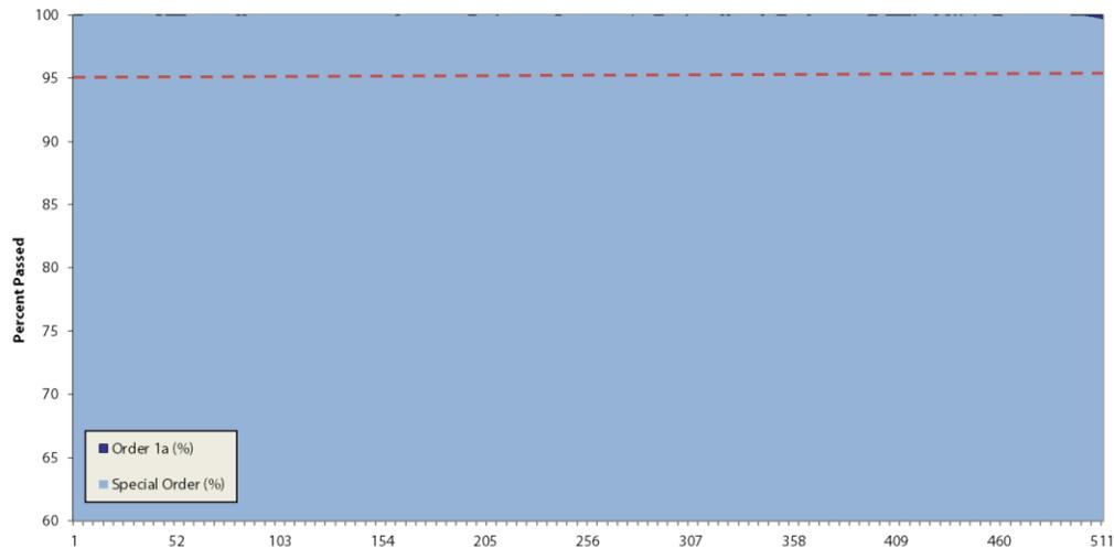
**Figure 2** Crossline analysis results for 2m bathymetric surface. Red dashed line indicates 95% confidence interval. Survey accuracy exceeds IHO Special Order standards.
