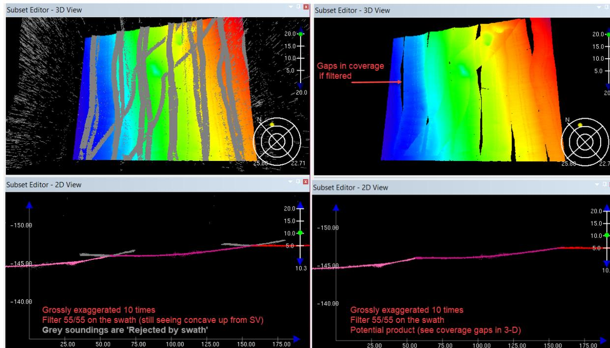
**Figure 7** Refraction artifacts in multibeam bathymetry. Top images are plan view; bottom images are across-track profile view. The refraction artifacts were mitigated by filtering each swath to remove the curved outer beams (shown in grey) caused by poor sound velocity modeling, however this was limited due to insufficient overlap which resulted in data gaps between swaths (top right).
