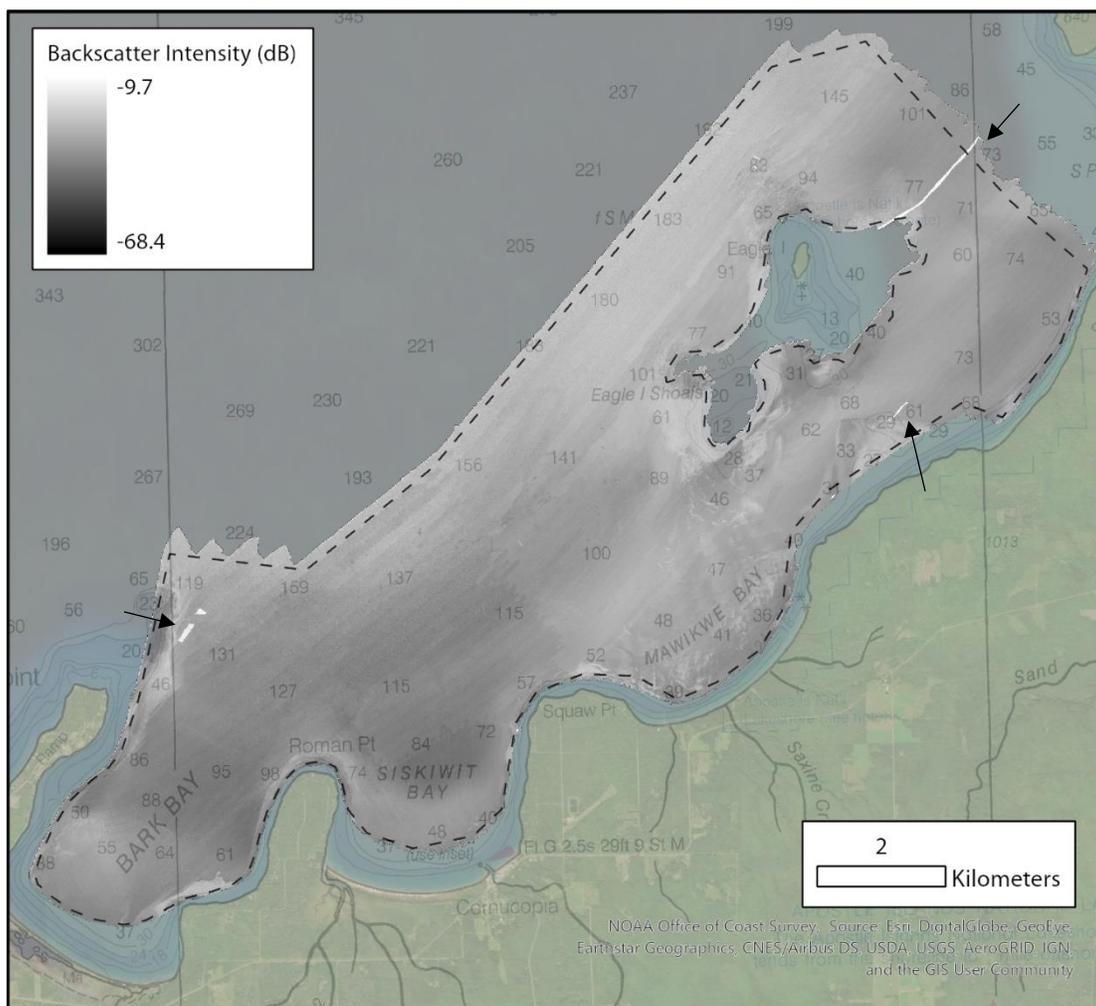
**Figure 4** Multibeam backscatter imagery mosaic (2m pixel resolution) for Areas 1-3. Black dashed line indicates boundary of survey area. Arrows indicate significant data gaps where no backscatter data was recorded (refer to section 4.1). Background is NOAA chart 14966 with soundings shown in feet relative to Lake Superior Low Water Datum (601.1 feet).
